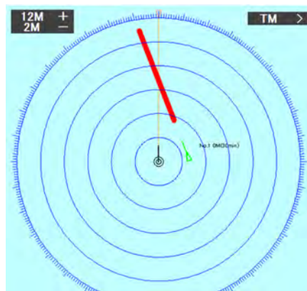
Fig.6.5 Encounter situation with a same course vessel at almost the same speed as the own ship on the starboard
